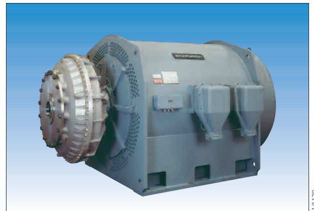
Shredder drive, 1,120 kW, 6.6 kV, 10-pole, star-delta starting, with turbo coupling
