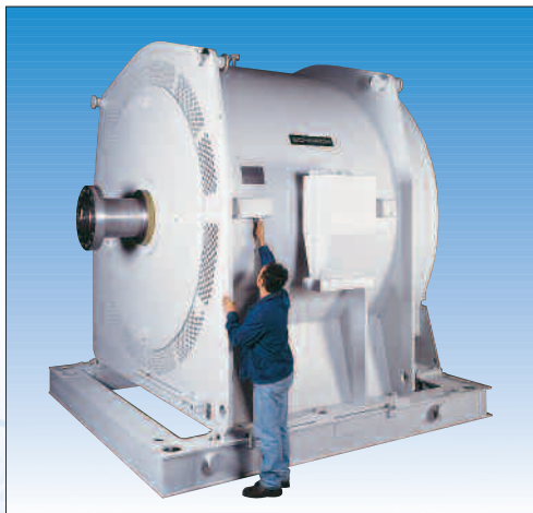
Piston compressor drive, 2,150 kW, 11 kV, 20-pole, IM D2
