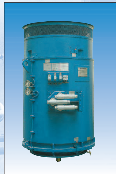
Pump drive, 600 kW, 6 kV, 2-pole, IM V1, connection via cable plugs
