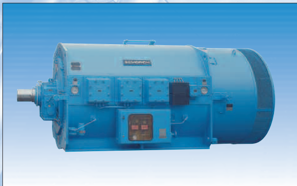
Pump drive, 3,500 kW, 6 kV, 4-pole, sleeve bearings with force-feed lubrication, Pressurized enclosure Exp
